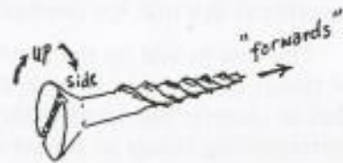
Right-handed helical screw
